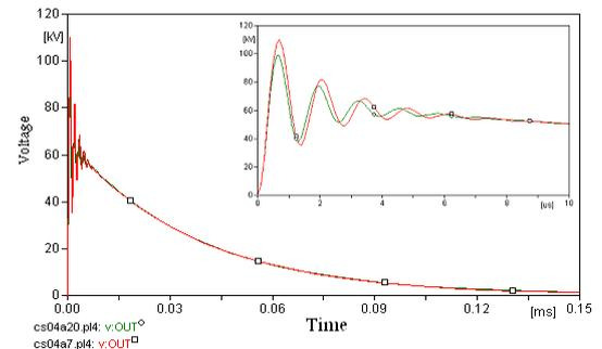
Fig.(10-a) Voltage wave form for CS04,  $a = 7$  and 20mm
