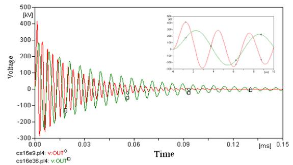
Fig.(7-a) Voltage wave form for CS16,  $\epsilon = 9$  and 36
