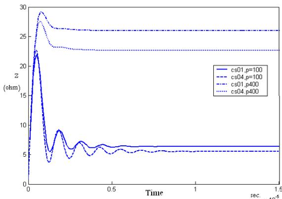
Fig.(3-a) Transient impedance for CS01 and CS04 grids for  $\rho=100,400 \Omega.m$
