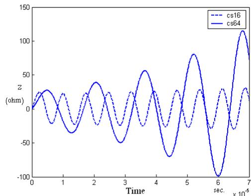
Fig.(2-b) Transient impedance for CS16 and CS64 grids
