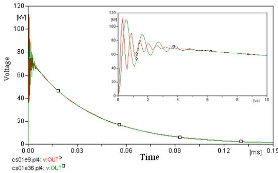
Fig.(5-a) Voltage wave form for CS01,  $\epsilon = 9$  and 36
