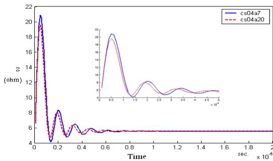
Fig.(10-b) Transient impedance for CS04,  $a=7$  and 20mm
