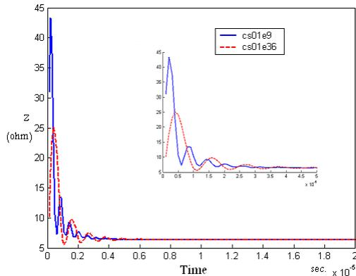
Fig.(5-b) Transient impedance for CS01,  $\epsilon = 9$  and 36
