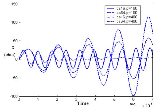
Fig.(3-b) Transient impedance for CS16 and CS64 grids for  $\rho=100,400 \Omega.m$
