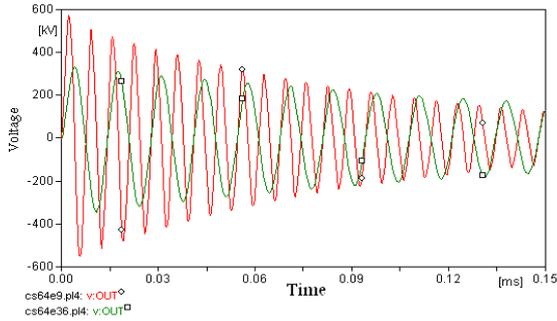
Fig.(8-a) Voltage wave form for CS64,  $\epsilon = 9$  and 36
