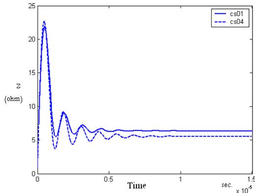
Fig.(2-a) Transient impedance for CS01 and CS04 grids
