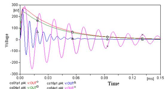
Fig.(4-b) Voltage wave form for  $\rho=400 \Omega.m$
