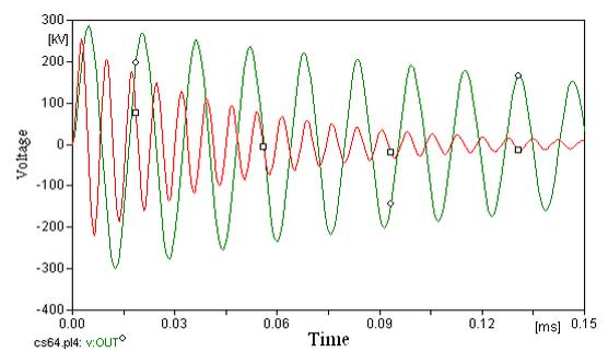
Fig.(2-d) Voltage wave form for CS16 and CS64 grids
