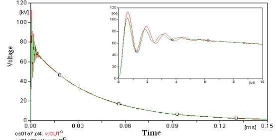
Fig.(9-a) Voltage wave form for CS01,  $a = 7$  and 20mm
