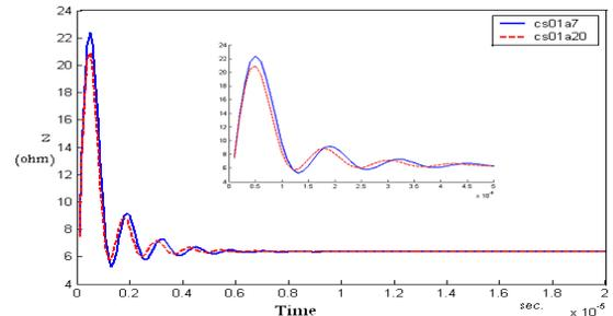
Fig.(9-b) Transient impedance for CS01,  $a = 7$  and 20mm
