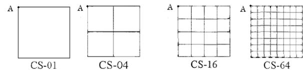
Fig.(1) Different number of meshes for square grids
