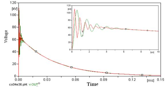
Fig.(6-a) Voltage wave form for CS04,  $\epsilon = 9$  and 36
