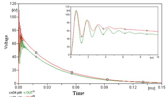
Fig.(2-c) Voltage wave form for CS01 and CS04 grids
